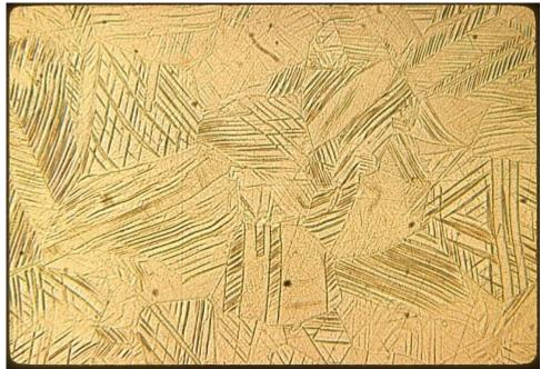
This is a phosphor bronze, shown at 200X at left and at 500X below. Phosphor bronze is copper that has been deoxidized with phosphorus. It is much harder and stronger than pure copper, because of the unconsumed phosphorus.
